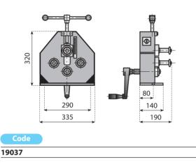
IMPORTANT: the bending machines are supplied without rollers, these must be ordered separately according to the guide rail type (see table).
